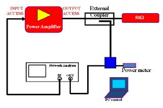
Figure 3 : Prana Test bench
