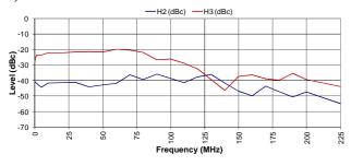
Figure 7 : Harmonic ratio @1 dB of compression
