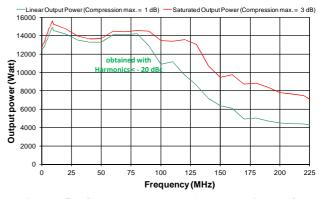
Figure 5 : Output power at 1 dB and 3 dB of compression
