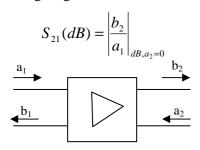
b<sub>2</sub>: transmitted wave at the output a<sub>1</sub>: incident wave at the input
